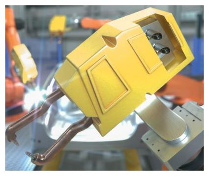
Monitoring the cooling circuit on welding clamps
